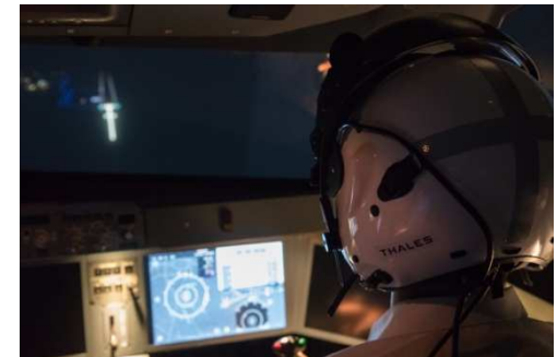
THALES HMD system in Generic Cockpit simulator at DLR in Braunschweig
