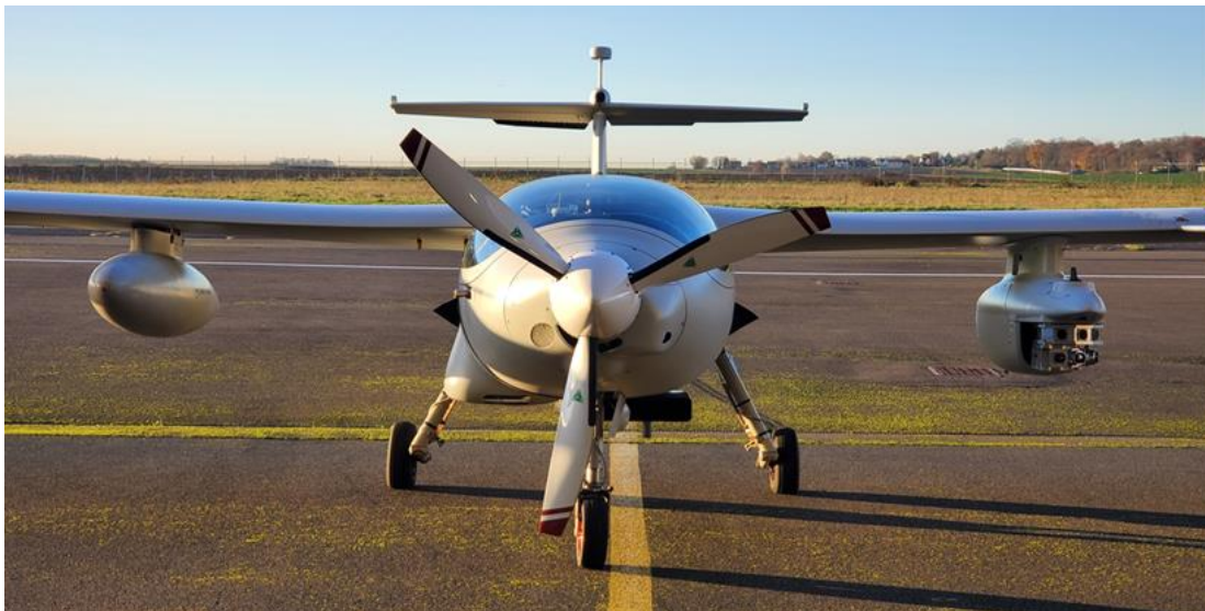
Integration of DAA function on an instrumentation POD on Patroller RPAS
