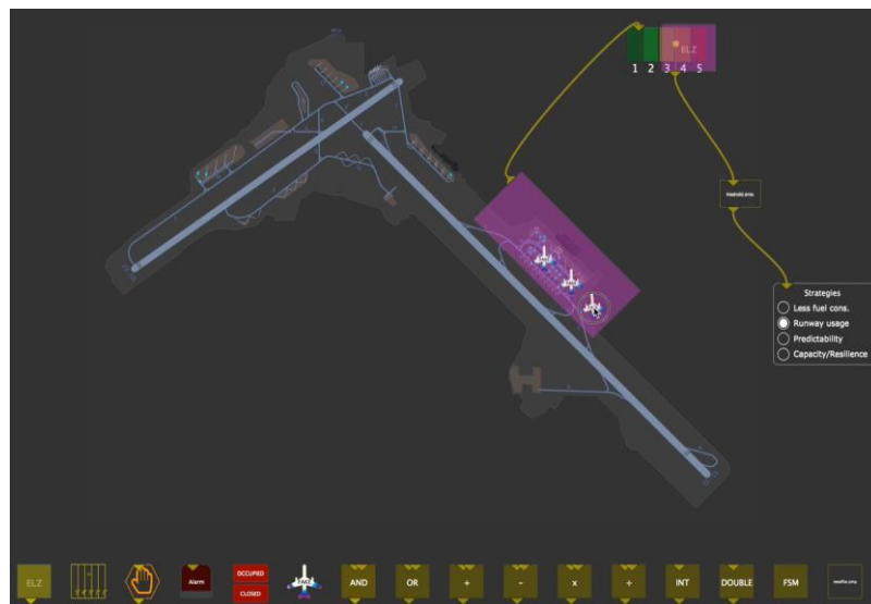
Figure 13 – Programming an automatic change of global strategy with the DSGL according to the number of flights at apron 9
