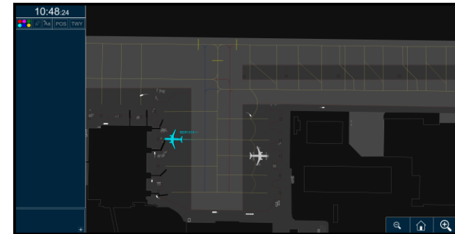
LiDAR GUI for the apron CWP
