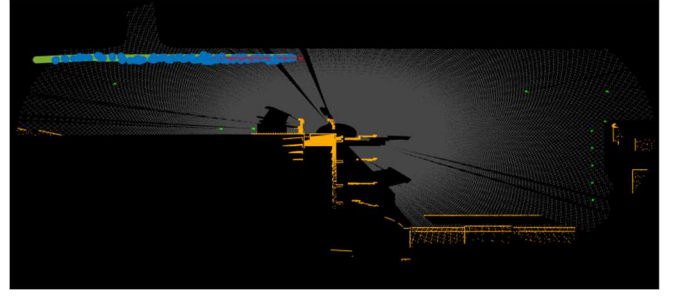
Figure 9. Bird's eye view of the tracked positions (blue) of a taxiing aircraft A320 (red points) along the ground-truth path (green) using Algorithm 1. See the text for details.
